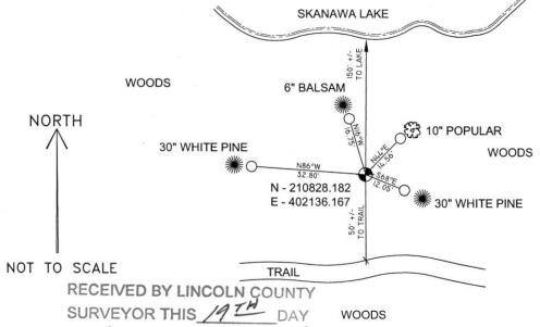
COORDINATES ARE REFERENCED TO THE LINCOLN COUNTY COORDINATE SYSTEM AS DEVELOPED BY THE WISCONSIN DEPARTMENT OF TRANSPORTATION AND ARE BASED ON GPS OBSERVATIONS TO CONTROL POINTS AS SUPPLIED BY LINCOLN COUNTY.
