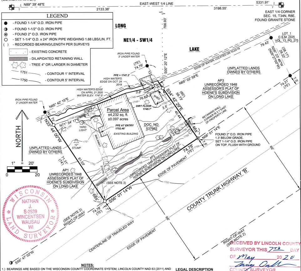
REFERENCED TO THE EAST-WEST 1/4 LINE OF SECTION 15, TOWNSHIP 34 NORTH, RANGE 8 EAST, MEASURED TO BEAR NORTH 89°39'48" EAST. ELEVATIONS ARE BASED ON NAVD 88 AND ARE REFERENCED TO NGS HEIGHT MOD POINT #DP1690 (FLEV. 1562.89')
