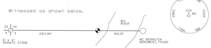
(c)(d)(e) Plan view of corner with ties to at least 4 witness monuments. If in disagreement with previously established corner, show the distances between the two corners and also indicate the ties to the disputed corner.
