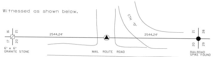
(c)(d)(e) Plan view of corner with ties to at least 4 witness monuments. If in disagreement with previously established corner, show the distances between the two corners and also indicate the ties to the disputed corner.
