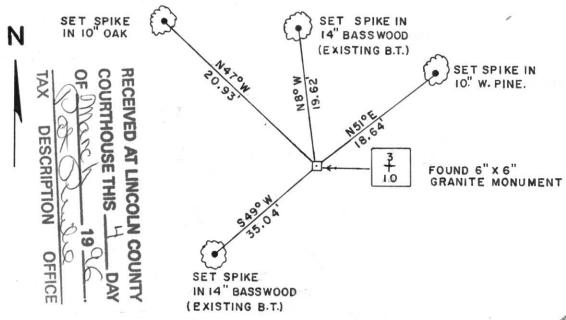
NOTE: TIES ARE TAKEN DIRECT BEARINGS TAKEN WITH A HANDHELD MAGNET COMPASS, NO SCALE.
