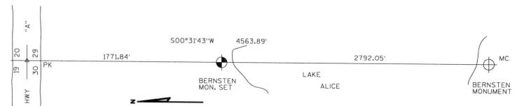
(c)(d)(e) Plan view of corner with ties to at least 4 witness monuments. If in disagreement with previously established corner, show the distances between the two corners and also indicate the ties to the disputed corner.
