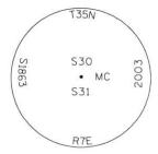
(c)(d)(e) Plan view of corner with ties to at least 4 witness monuments. If in disagreement with previously established corner, show the distances between the two corners and also indicate the ties to the disputed corner.
