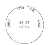
(c)(d)(e) Plan view of corner with ties to at least 4 witness monuments. If in disagreement with previously established corner, show the distances between the two corners and also indicate the ties to the disputed corner.
