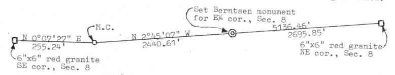
c) (d) (e) Plan view of corner with ties to at least 4 witness monuments. If in disagreement with previously established corner, show the distances between the two corners and also indicate the ties to the disputed corner.
