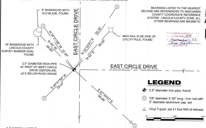
A-E 7.08(3)(e) 1865 Surveyor set a post, 1978 Surveyor found an iron pipe, 2013 Surveyor found a 2 1/2" o.d. iron pipe. I found a 2.5" diameter iron pipe.
