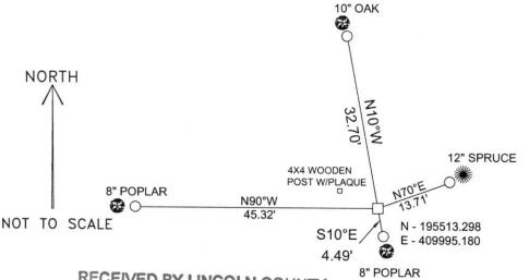
COORDINATES ARE REFERENCED TO THE LINCOLN COUNTY COORDINATE SYSTEM AS DEVELOPED BY THE WISCONSIN DEPARTMENT OF TRANSPORTATION AND WERE DETERMINED BY GPS OBSERVATIONS ON CONTROL POINTS AS SUPPLIED BY LINCOLN COUNTY.
