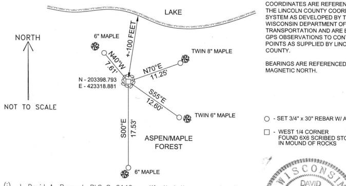
COORDINATES ARE REFERENCED TO THE LINCOLN COUNTY COORDINATE SYSTEM AS DEVELOPED BY THE WISCONSIN DEPARTMENT OF TRANSPORTATION AND ARE BASED ON GPS OBSERVATIONS TO CONTROL POINTS AS SUPPLIED BY LINCOLN
