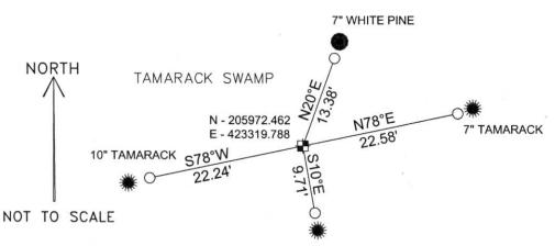
COORDINATES ARE REFERENCED TO THE LINCOLN COUNTY COORDINATE SYSTEM AS DEVELOPED BY THE WISCONSIN DEPARTMENT OF TRANSPORTATION AND ARE BASED ON GPS OBSERVATIONS TO CONTROL POINTS AS SUPPLIED BY LINCOLN COUNTY.
