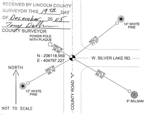
COORDINATES ARE REFERENCED TO THE LINCOLN COUNTY COORDINATE SYSTEM AS DEVELOPED BY THE WISCONSIN DEPARTMENT OF TRANSPORTATION AND ARE BASED ON GPS OBSERVATIONS TO CONTROL POINTS AS SUPPLIED BY LINCOLN COUNTY.
