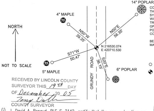
COORDINATES ARE REFERENCED TO THE LINCOLN COUNTY COORDINATE SYSTEM AS DEVELOPED BY THE WISCONSIN DEPARTMENT OF TRANSPORTATION AND ARE BASED ON GPS OBSERVATIONS TO CONTROL POINTS AS SUPPLIED BY LINCOLN COUNTY.
