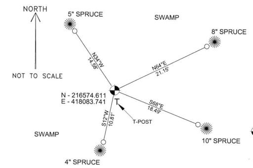
COORDINATES ARE REFERENCED TO THE LINCOLN COUNTY COORDINATE SYSTEM AS DEVELOPED BY THE WISCONSIN DEPARTMENT OF TRANSPORTATION AND ARE BASED ON GPS OBSERVATIONS TO CONTROL POINTS AS SUPPLIED BY LINCOLN COUNTY.
