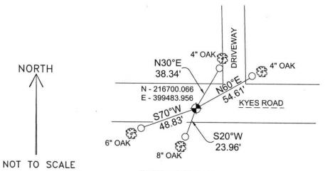
COORDINATES ARE REFERENCED TO THE LINCOLN COUNTY COORDINATE SYSTEM AS DEVELOPED BY THE WISCONSIN DEPARTMENT OF TRANSPORTATION AND ARE BASED ON GPS OBSERVATIONS TO CONTROL POINTS AS SUPPLIED BY LINCOLN COUNTY
