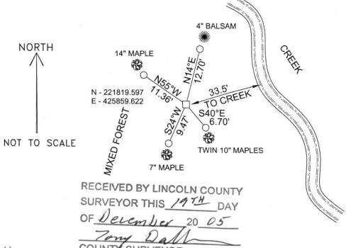
COORDINATES ARE REFERENCED TO THE LINCOLN COUNTY COORDINATE SYSTEM AS DEVELOPED BY THE WISCONSIN DEPARTMENT OF TRANSPORTATION AND ARE BASED ON GPS OBSERVATIONS TO CONTROL POINTS AS SUPPLIED BY LINCOLN COUNTY.
