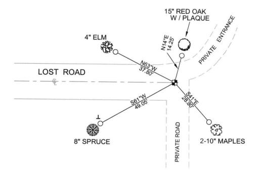
COORDINATES ARE REFERENCED TO THE LINCOLN COUNTY COORDINATE SYSTEM AS DEVELOPED BY THE WISCONSIN DEPARTMENT OF TRANSPORTATION AND WERE DETERMINED BY GPS OBSERVATIONS ON CONTROL POINTS AS SUPPLIED BY LINCOLN COUNTY.
