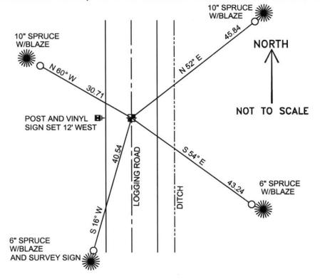
COORDINATES ARE REFERENCED TO THE LINCOLN COUNTY COORDINATE SYSTEM AS DEVELOPED BY THE WISCONSIN DEPARTMENT OF TRANSPORTATION AND WERE DETERMINED BY GPS OBSERVATIONS ON CONTROL POINTS AS SUPPLIED BY LINCOLN COUNTY.
