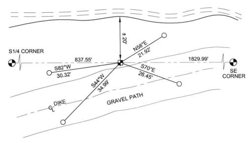
COORDINATES ARE REFERENCED TO THE LINCOLN COUNTY COORDINATE SYSTEM AS DEVELOPED BY THE WISCONSIN DEPARTMENT OF TRANSPORTATION AND WERE DETERMINED BY GPS OBSERVATIONS ON CONTROL POINTS AS SUPPLIED BY LINCOLN COUNTY.
