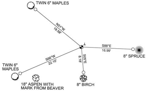
COORDINATES ARE REFERENCED TO THE LINCOLN COUNTY COORDINATE SYSTEM AS DEVELOPED BY THE WISCONSIN DEPARTMENT OF TRANSPORTATION AND WERE DETERMINED BY GPS OBSERVATIONS ON CONTROL POINTS AS SUPPLIED BY LINCOLN COUNTY.
