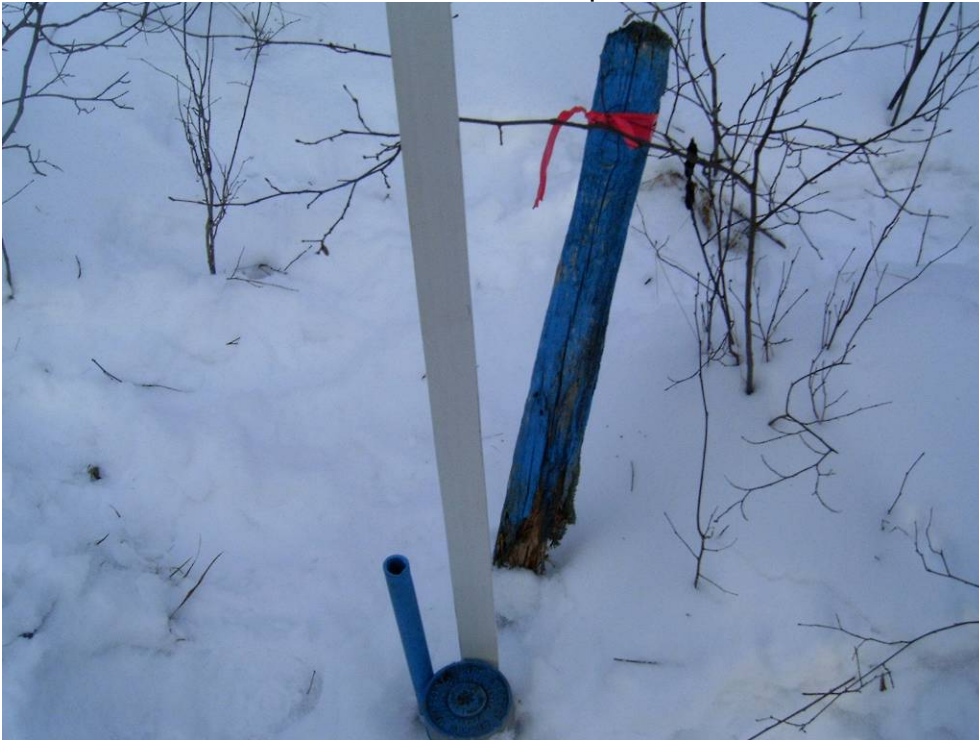
Picture 6 –Found Berntsen, 1 Inch Iron Pipe and Wood Post
