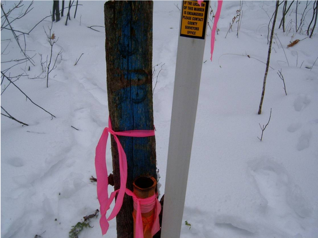
Picture 5 –Found 1” Iron Pipe with Wood Post at Corner
