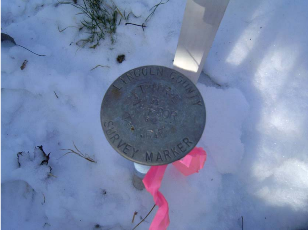
Picture 5 –Found 1.0 Aluminum Pipe with Stamped Cap at Corner
