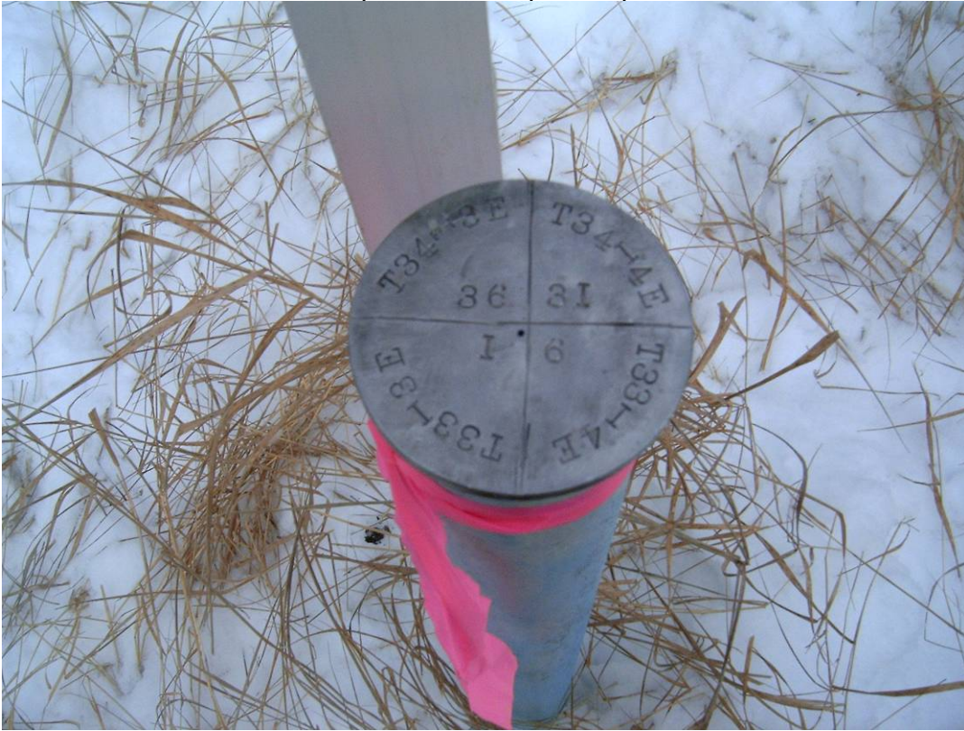
Picture 5 –Found 2.0 Iron Pipe with Stamped Cap at Corner
