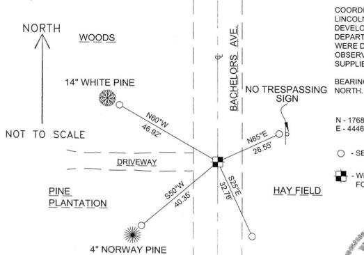
COORDINATES ARE REFERENCED TO THE LINCOLN COUNTY COORDINATE SYSTEM AS DEVELOPED BY THE WISCONSIN DEPARTMENT OF TRANSPORTATION AND WERE DETERMINED BY GPS OBSERVATIONS ON CONTROL POINTS AS SUPPLIED BY LINCOLN COUNTY.
