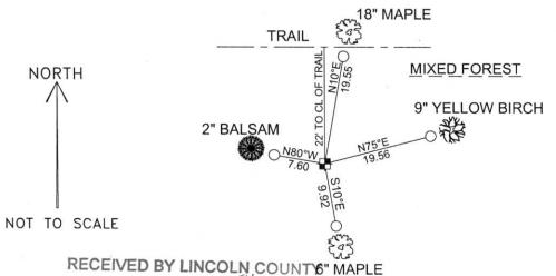
COORDINATES ARE REFERENCED TO THE LINCOLN COUNTY COORDINATE SYSTEM AS DEVELOPED BY THE WISCONSIN DEPARTMENT OF TRANSPORTATION AND WERE **DETERMINED BY GPS OBSERVATIONS** ON CONTROL POINTS AS SUPPLIED BY LINCOLN COUNTY.
