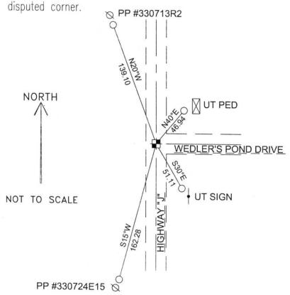
COORDINATES ARE REFERENCED TO THE LINCOLN COUNTY COORDINATE SYSTEM AS DEVELOPED BY THE WISCONSIN DEPARTMENT OF TRANSPORTATION AND WERE DETERMINED BY GPS OBSERVATIONS ON CONTROL POINTS AS SUPPLIED BY LINCOLN COUNTY.
