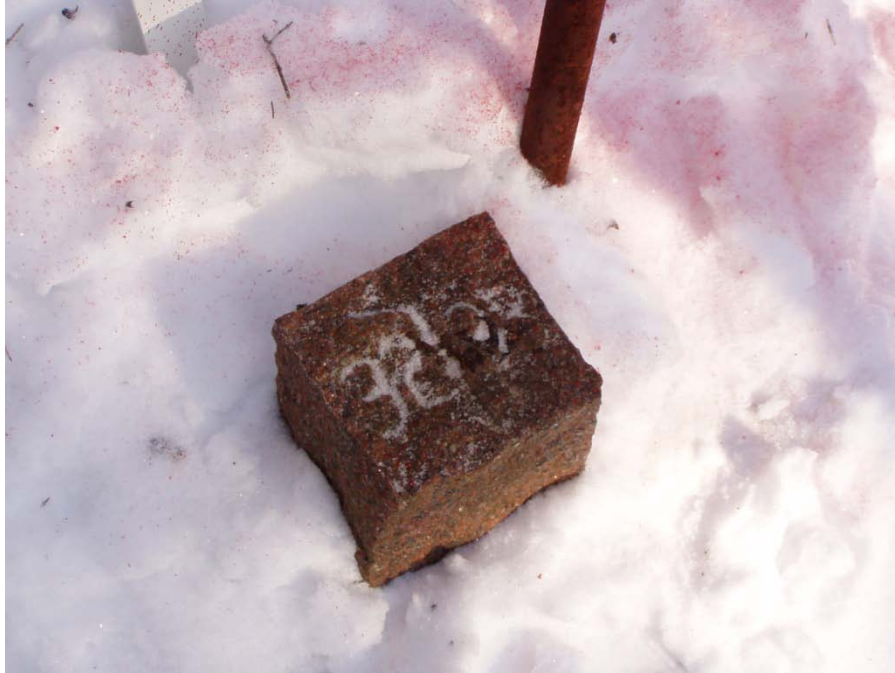
WEST ¼ CORNER, SECTION 33 – 6" SQUARE GRANITE STONE FOUND
