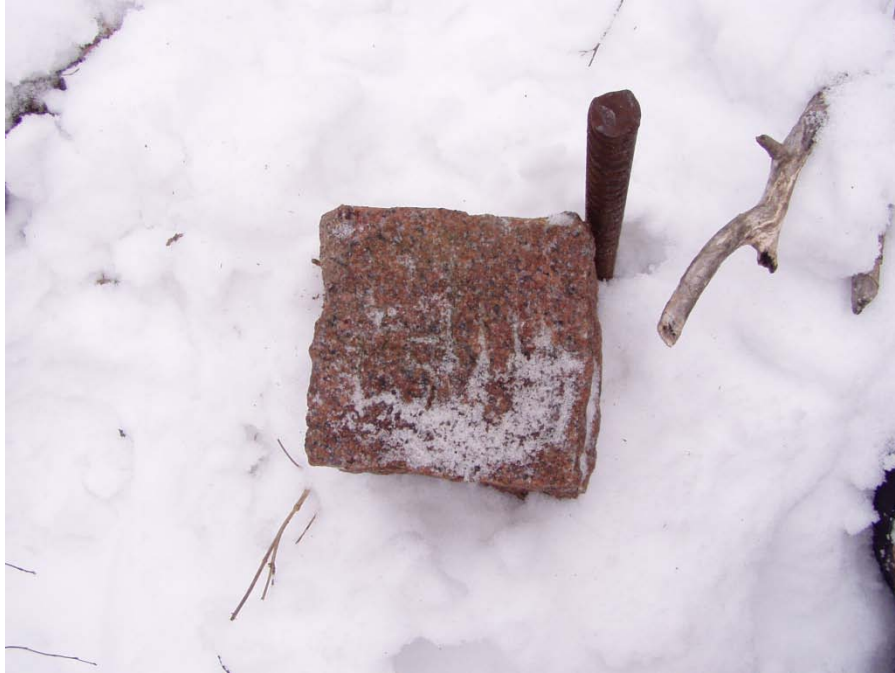
EAST ¼ CORNER, SECTION 15 – 6" SQUARE GRANITE STONE FOUND
