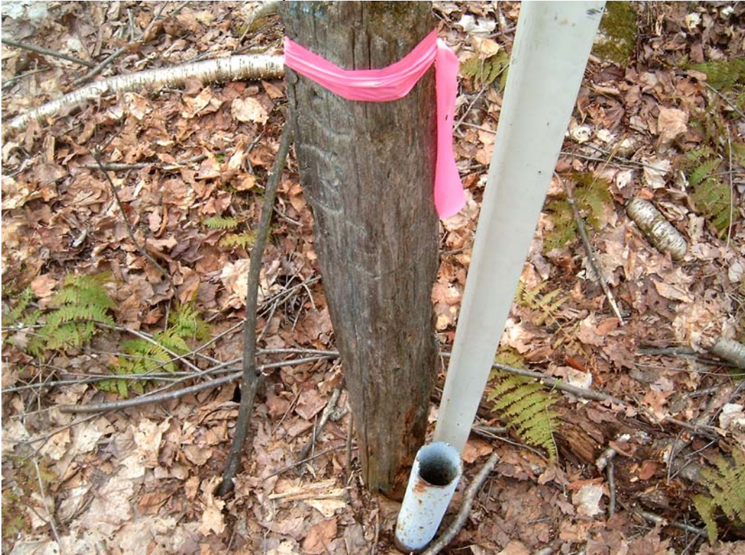
Picture 5 –Found 2.0 Iron Pipe with Wood Post at corner
