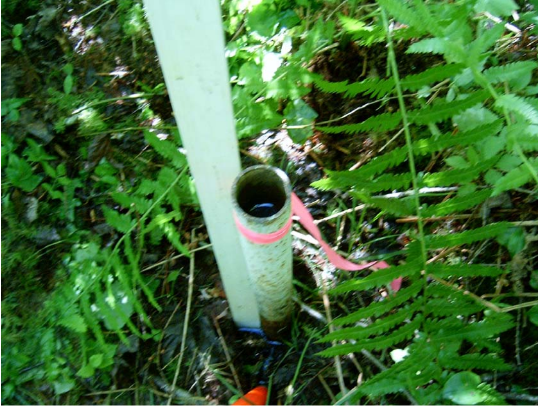
Picture 5 –Found 1.5 Iron Pipe at Corner
