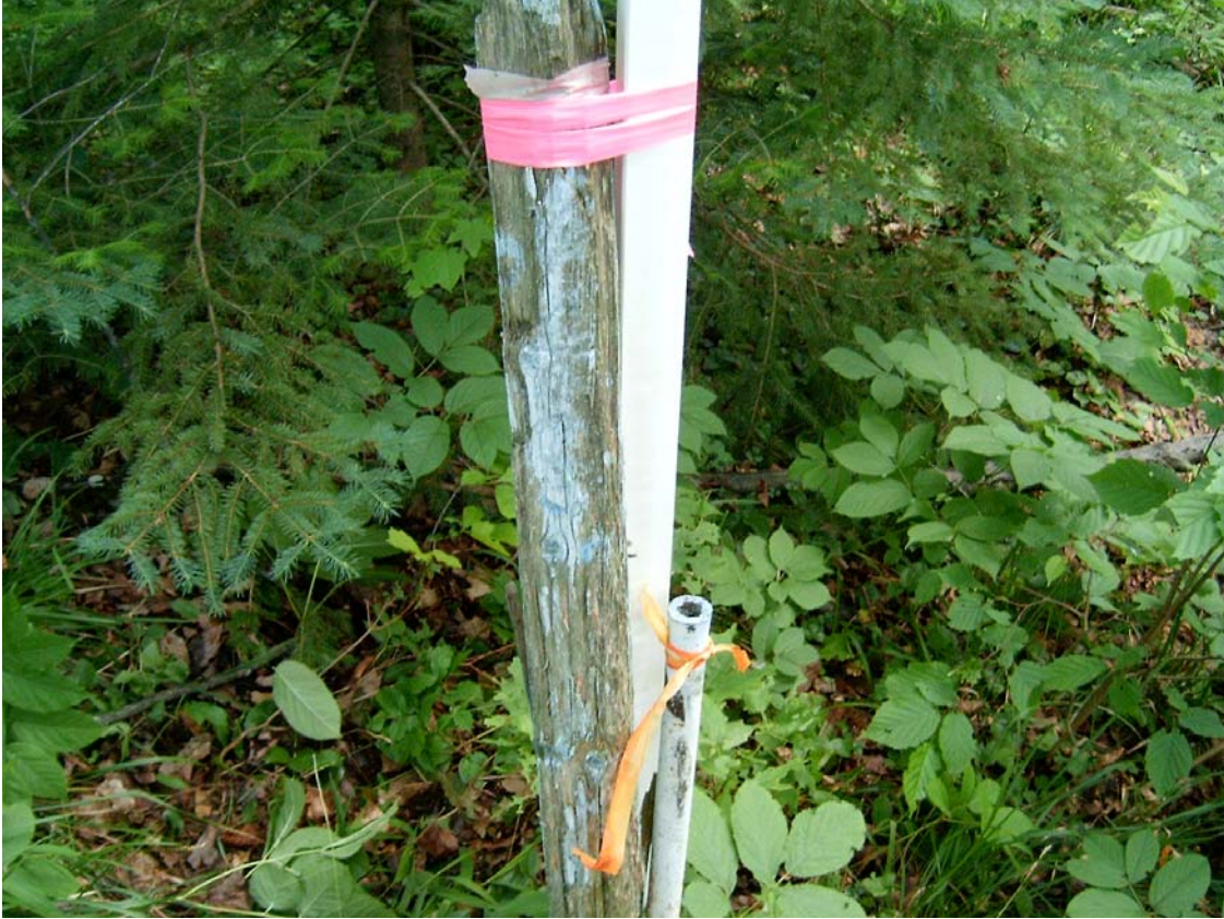
Picture 5 –Found 1.0 Iron Pipe and Wood Post at Corner
