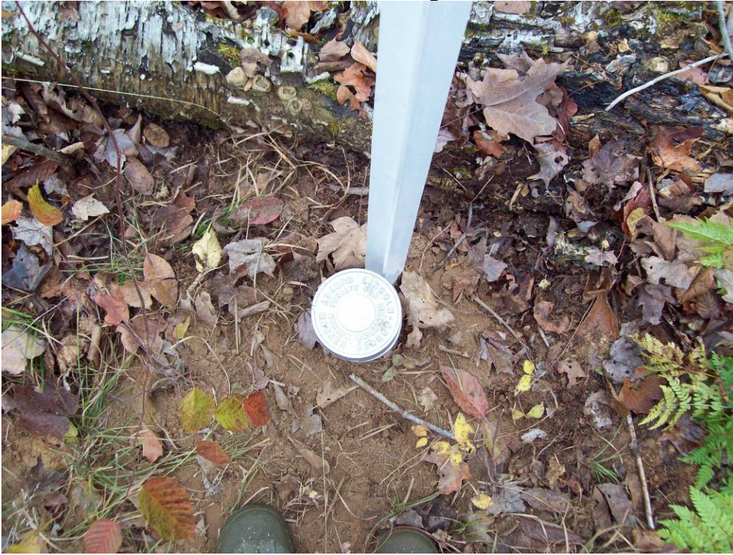
Picture 5 –Set Bernsten Monument and Sign at Corner
