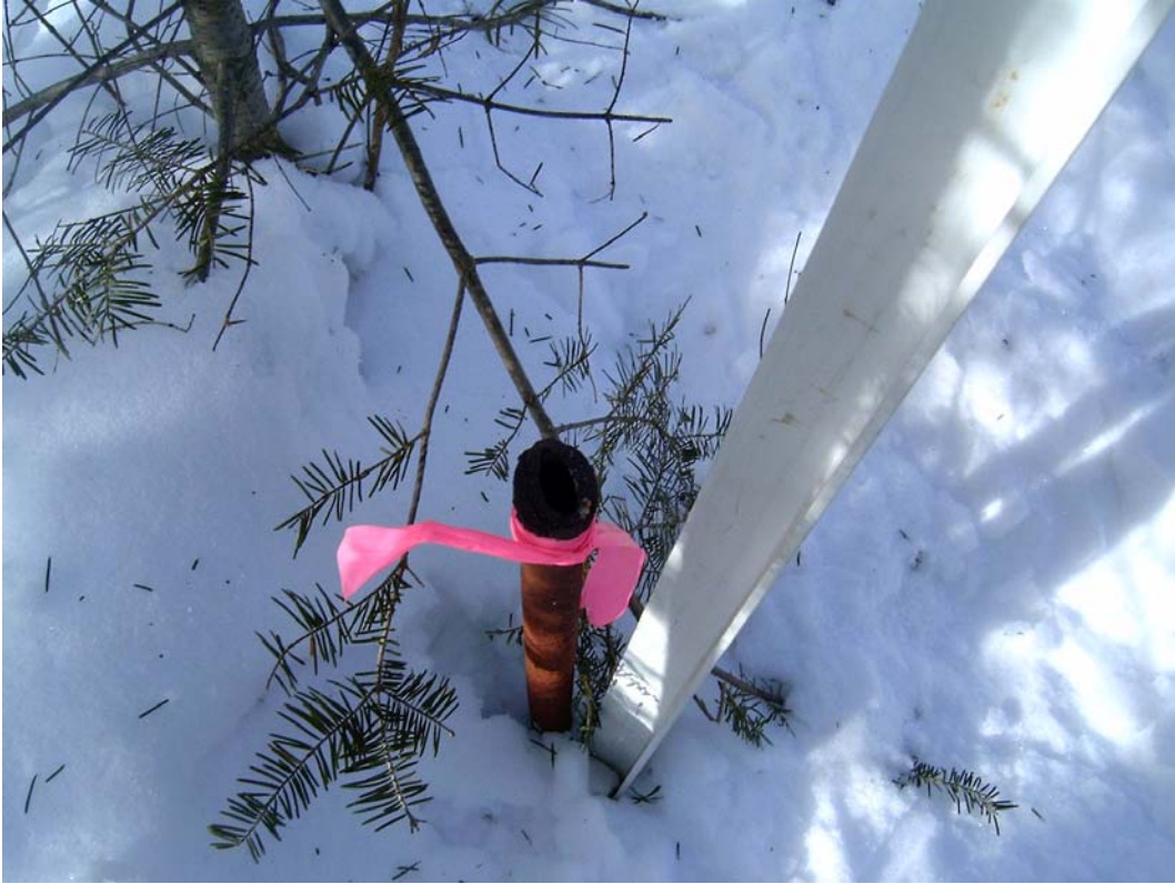
Picture 5 –Found 1 Inch Iron Pipe at Corner
