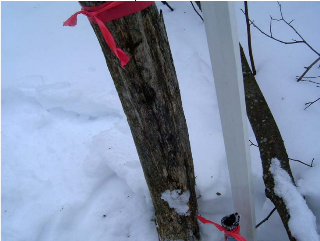
Picture 6 –Found 1 Inch Iron Pipe and Wood Post at Corner
