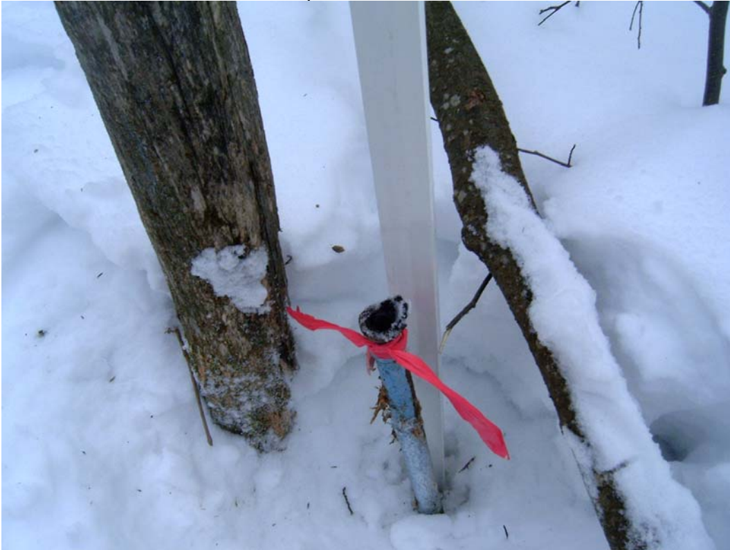
Picture 5 –Found 1 Inch Iron Pipe and Wood Post at Corner
