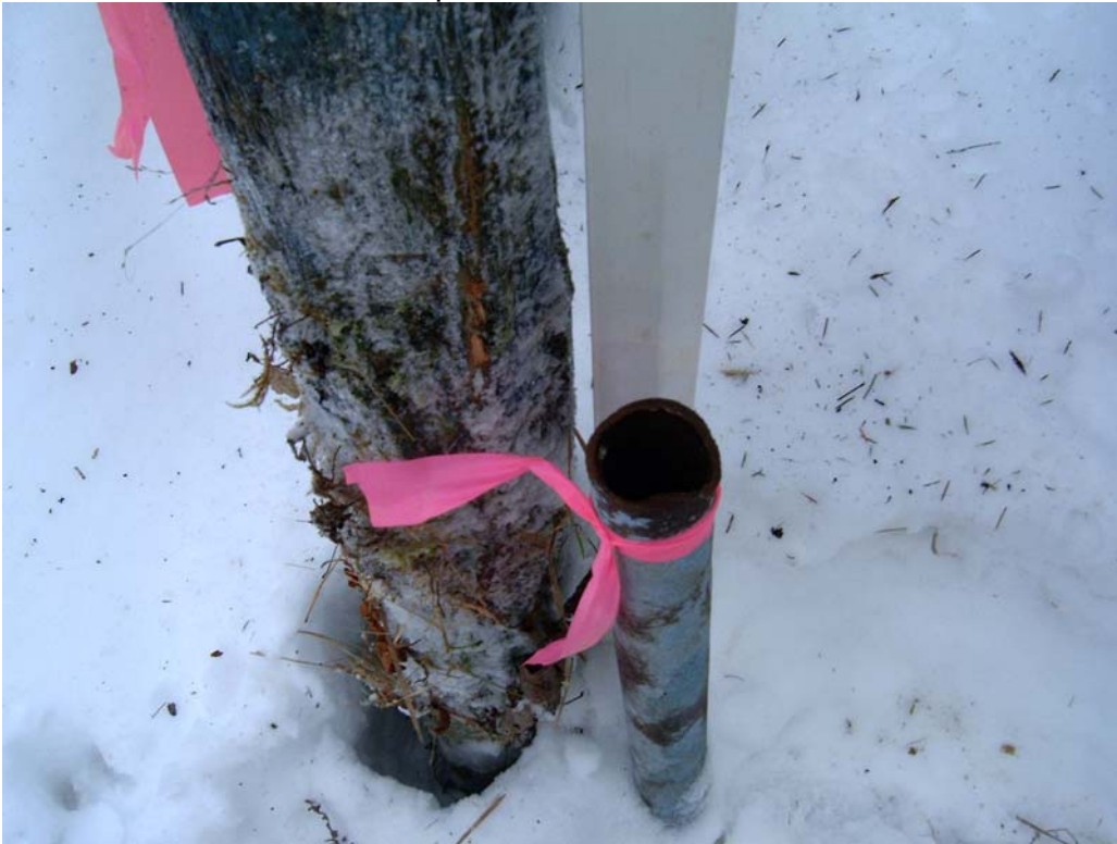
Picture 5 –Found 1.5 Iron Pipe and Wood Post at Corner
