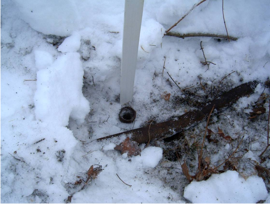
Picture 5 –Found 1.5 Iron Pipe at Corner
