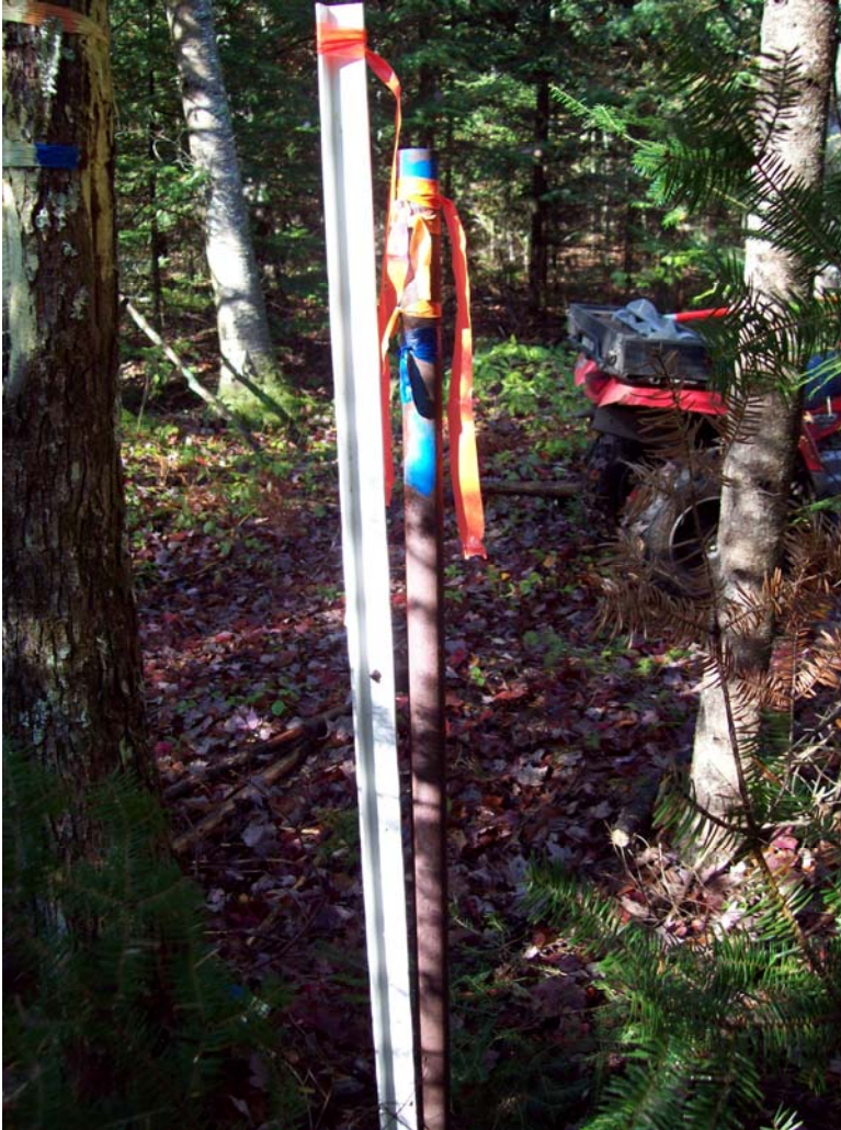
Picture 5 – Found 1.5" Iron Pipe, Set Sign
