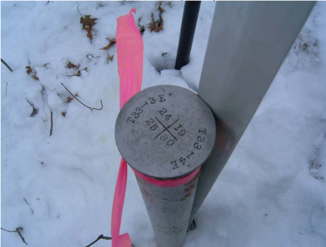
Picture 5 –Found 2.0 Iron Pipe with Stamped Cap at corner
