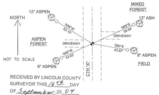
COORDINATES ARE REFERENCED TO THE LINCOLN COUNTY COORDINATE SYSTEM AS DEVELOPED BY THE WISCONSIN DEPARTMENT OF TRANSPORTATION AND WERE DETERMINED BY GPS OBSERVATIONS ON CONTROL POINTS AS SUPPLIED BY LINCOLN COUNTY.
