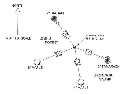
COORDINATES ARE REFERENCED TO THE LINCOLN COUNTY COORDINATE SYSTEM AS DEVELOPED BY THE WISCONSIN DEPARTMENT OF TRANSPORTATION AND WERE DETERMINED BY GPS OBSERVATIONS ON CONTROL POINTS AS SUPPLIED BY LINCOLN COUNTY.
