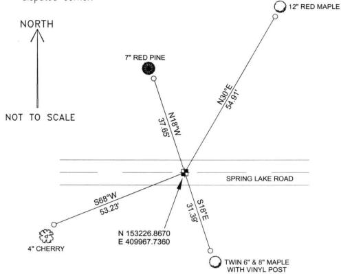
COORDINATES ARE REFERENCED TO THE LINCOLN COUNTY COORDINATE SYSTEM AS DEVELOPED BY THE WISCONSIN DEPARTMENT OF TRANSPORTATION AND WERE DETERMINED BY GPS OBSERVATIONS ON CONTROL POINTS AS SUPPLIED BY LINCOLN COUNTY.
