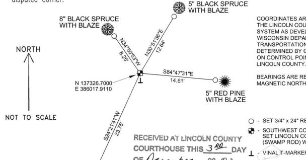
COORDINATES ARE REFERENCED TO THE LINCOLN COUNTY COORDINATE SYSTEM AS DEVELOPED BY THE WISCONSIN DEPARTMENT OF TRANSPORTATION AND WERE **DETERMINED BY GPS OBSERVATIONS** ON CONTROL POINTS AS SUPPLIED BY
