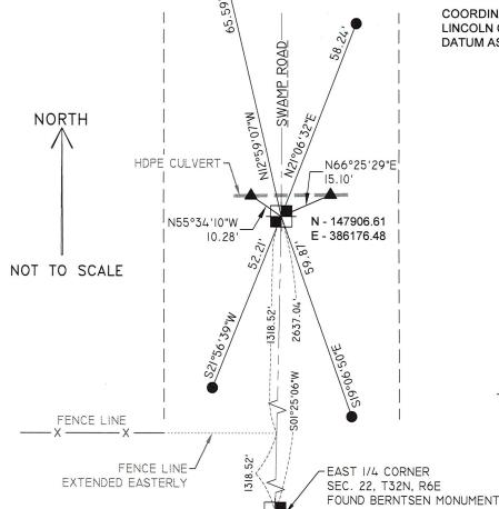
COORDINATES AND BEARINGS ARE BASED ON THE LINCOLN COUNTY COORDINATE SYSTEM, NAD 83(2011) DATUM AS ESTABLISHED BY THE WISCORS NETWORK.
