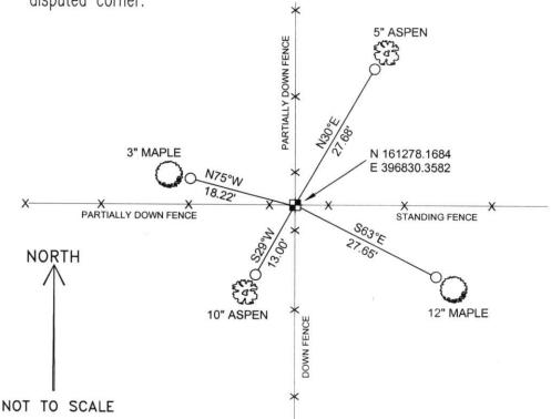
COORDINATES ARE REFERENCED TO THE LINCOLN COUNTY COORDINATE SYSTEM AS DEVELOPED BY THE WISCONSIN DEPARTMENT OF TRANSPORTATION AND WERE DETERMINED BY GPS OBSERVATIONS ON CONTROL POINTS AS SUPPLIED BY LINCOLN COUNTY.
