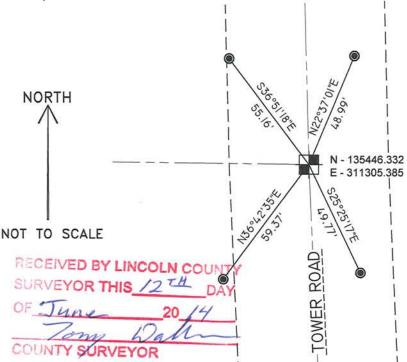
BEARINGS AND COORDINATES ARE BASED ON THE LINCOLN COUNTY COORDINATE SYSTEM NAD 83(2011) DATUM.
