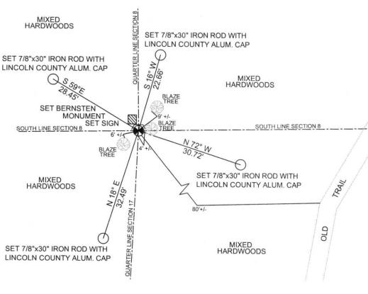
COORDINATES ARE REFERENCED TO LINCOLN COUNTY COORDINATE SYSTEM AS DEVELOPED BY THE WI. DEPARTMENT OF TRANSPORTATION AND ARE BASED ON GPS OBSERVATIONS TO CONTROL POINTS AS SUPPLIED BY LINCOLN COUNTY
