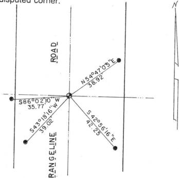
All ties to 7/8" x 30" Iron Re-bars with caps. Special County Witness post alongside one of the ties. From the NE Cor. to  $E_4^{\prime}$  Cor. S0 10'26"W, 2632.53'. From the NE Cor. to  $N_4^{\prime}$  Cor. S89 45'26"W, 2678.60'
